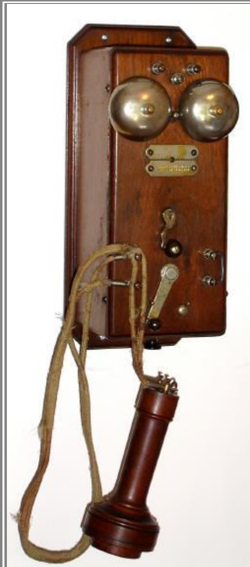
The "Coffin" was probably the most famous telephone produced by Williams. A single magneto hand telephone could serve as both a receiver and transmitter. Some models came with two, one for each hand. Coffin images courtesy of Tom Adams
