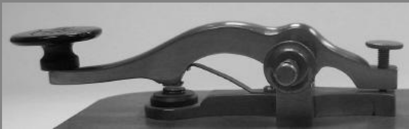
A Hinds and Williams telegraph key and an advertisement from 1856. (Key courtesy of Gil Schlehman, K9WDY)
