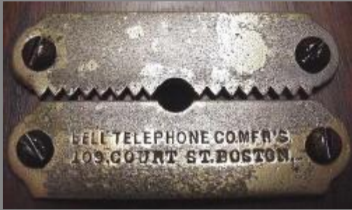
A close-up view of the "Coffin's" markings. The two plates also served as a lightning arrester.
