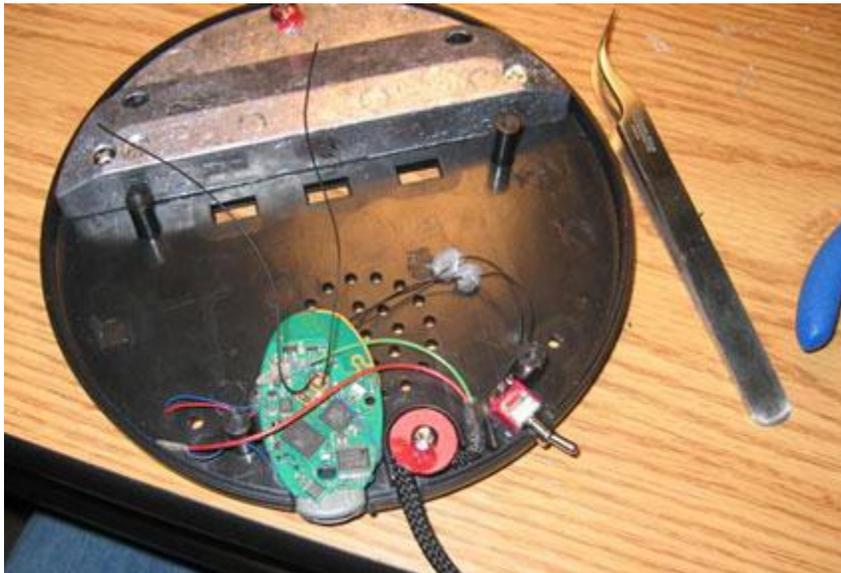
4. Interface the main button contacts with a modified version of the existing arm-switch. The main button requires a ?pulse-like? connection. We'd like this to happen whenever the speaker is lifted or put back. to get a rising and falling edge. Here's an ascii diagram:
