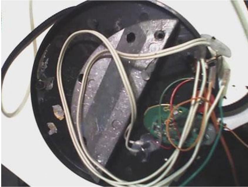
8. Mounting the clock is a serious pain in the ass. The clock I picked up at a craft store was a bit small for the dialpad. Make a mount from a mini cd. Tape one side of the CD, trace out the back of the clock, and dremel out the middle. Spray paint it black.
